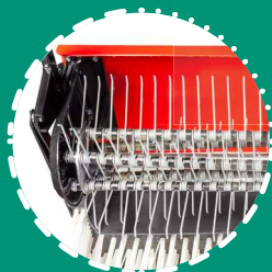
SPRING ROTOR independent activation 80 cm - 142 rpm
